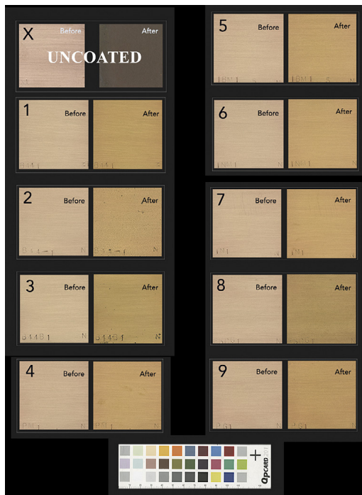
Figure 2. Scans of the coupons grouped to show before ageing (left) and after ageing (right)
